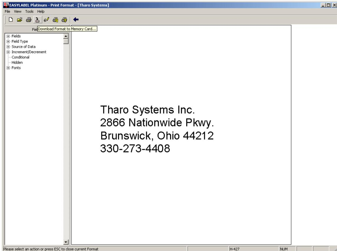
\*When the Download Format To Memory Card window opens you can choose a name for your downloaded format; whether you want to create a copy of the format as a text file; how the quantity to print will be handled and to which printer the format will be downloaded. After making your choices click OK and the download process will begin.
